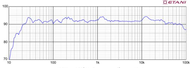
10Hz ~ 100kHz Frequency Characteristics
